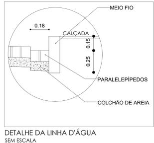
DETALHE DA LINHA D'ÁGUA SEM ESCALA
